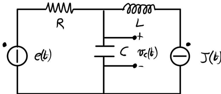
$$\begin{aligned} R &= 10 \Omega \\ C &= 10 \mu\text{F} \\ L &= 10 \text{ mH} \\ e(t) &= 20 \text{ V} \end{aligned}$$
