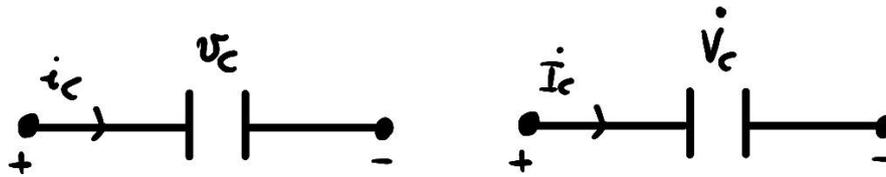
$$v_c(t) = \frac{1}{C} \int_{-\infty}^t i_c(\tau) d\tau \Rightarrow \dot{V}_c = \frac{1}{j\omega C} I_c = \frac{1}{j} \cdot \frac{1}{\omega C} I_M e^{j\phi_1} = -j \frac{1}{\omega C} I_M e^{j\phi_1} = e^{-j\frac{\pi}{2}} \frac{1}{\omega C} I_M e^{j\phi_1} = \frac{I_M}{j\omega C} e^{j(\phi_1 - \frac{\pi}{2})}$$
