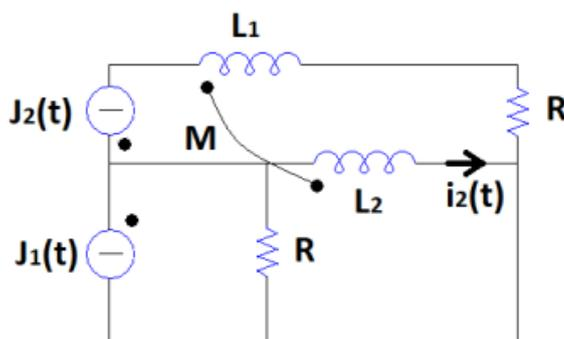
$$\begin{aligned} J_1(t) &= \sqrt{2} \sin(1000t) \text{ A}; \\ J_2(t) &= 2\sqrt{2} \sin(1000t + \pi/2) \text{ A}; \\ R &= 10 \Omega; \\ L_1 &= 10 \text{ mH}; \\ L_2 &= 20 \text{ mH}; \\ M &= 14 \text{ mH}. \end{aligned}$$
