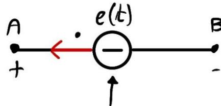
$$\begin{aligned} v_{AB}(t) &= e(t) \\ v_{BA}(t) &= -e(t) \end{aligned}$$
