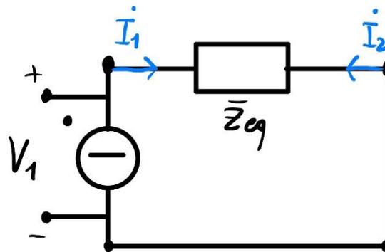
$$\bar{z}_{eq} = \frac{j\omega(L_2 - M) \cdot (R + j\omega M)}{j\omega(L_2 - M) + R + j\omega M}$$
