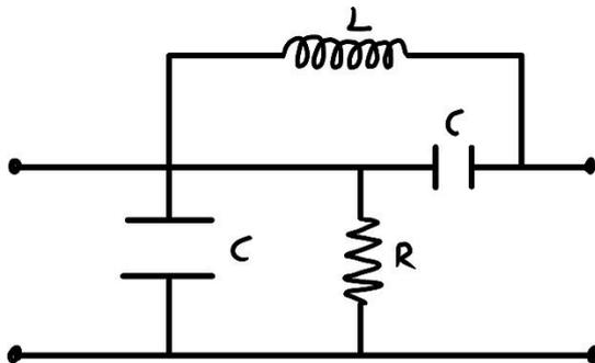
$$\begin{aligned} R &= 10 \Omega \\ L &= 10 \text{ mH} \\ C &= 10 \mu\text{F} \\ \omega &= 1000 \text{ rad/s} \end{aligned}$$
