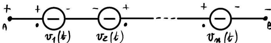
$$v_{AB}(t) = v_1(t) - v_2(t) + \dots + v_n(t)$$
