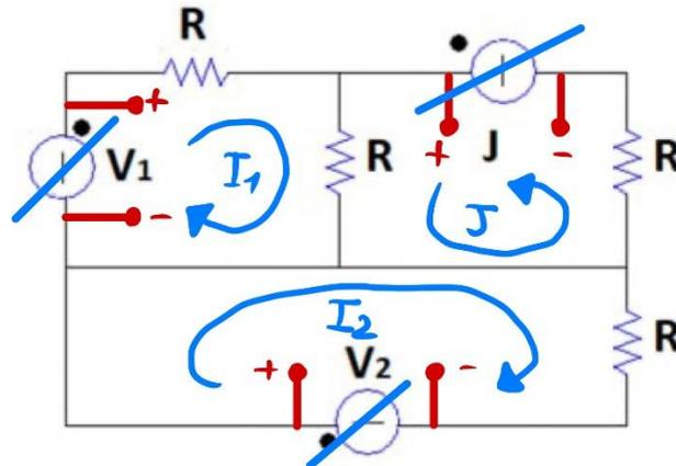
$$I_1: -V_1 + R \cdot I_1 + R \cdot (I_1 + J) = 0 \rightarrow -V_1 + 2R \cdot I_1 + R \cdot J = 0 \rightarrow I_1 = \frac{V_1 - R \cdot J}{2R} = -1 \text{ A}$$
