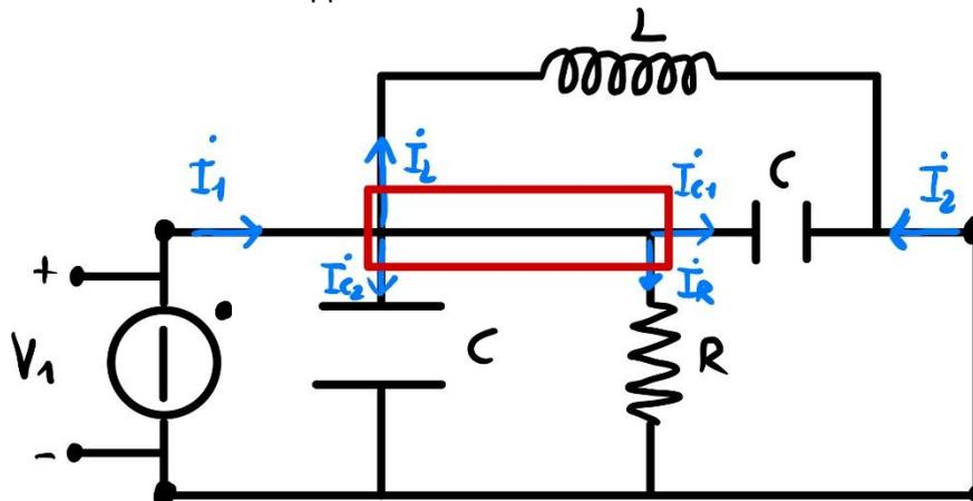
$$\begin{aligned} I_1 &= I_L + I_{C2} + I_{C1} + I_R = V_1 \left( \frac{1}{j\omega L} \right) + V_1 \left( \frac{1}{R} \right) + V_1(j\omega C) + V_1(j\omega C) = \\ &= V_1 \left( \frac{1}{j\omega L} + \frac{1}{R} + 2j\omega C \right) \end{aligned}$$
