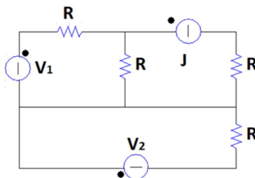
$$\begin{aligned} V_1 &= 10 \text{ V}; \\ V_2 &= 20 \text{ V} \\ J &= 3 \text{ A}; \\ R &= 10 \Omega; \end{aligned}$$
