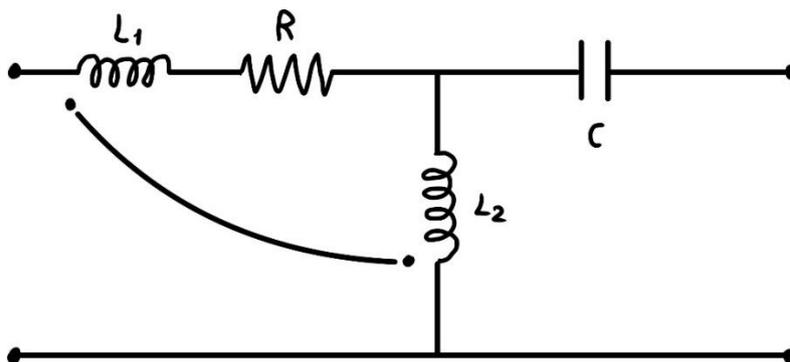
$$\begin{aligned}L_1 &= 20 \text{ mH} \\ L_2 &= 20 \text{ mH} \\ M &= 15 \text{ mH}\end{aligned}$$
