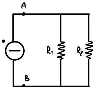
$$i_1 = \frac{G_1}{G_1 + G_2} J(t) = \frac{\frac{1}{R_1}}{\frac{1}{R_1} + \frac{1}{R_2}} J(t) = \frac{R_2}{R_1 + R_2} J(t)$$
