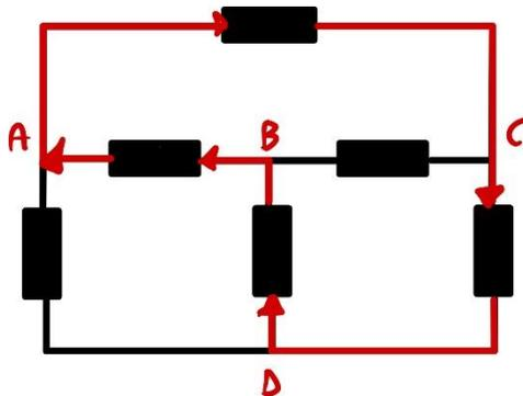
$$v_{AC}(t) + v_{CD}(t) + v_{DB}(t) + v_{BA}(t) = 0$$
