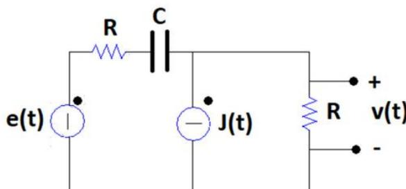
$$\begin{aligned} e(t) &= 50\sqrt{2} \sin(1000t) \text{ V}; \\ J(t) &= 2\sqrt{2} \cos(1000t) \text{ A}; \\ R &= 10 \Omega; \\ C &= 100 \mu\text{F}; \end{aligned}$$
